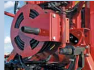
External cleaning Hose reel with 20 m hose and spray guns. The sprayer can be cleaned in the field.
