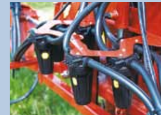
In-Line filters Extra filters built in the feed hoses.
