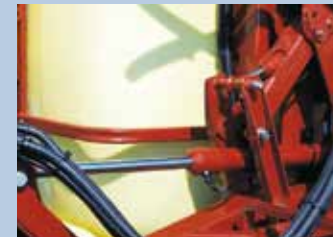
Hydraulic boom slant Extra double-acting hydraulic cylinder to correct boom position on slopes.
