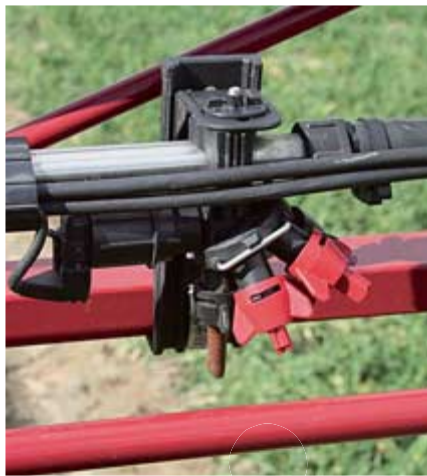
Multiple nozzle bodies (left) are operated electrically but rotated manually. The boom (below) uses three ultrasonic sensors for automatic boom control.
