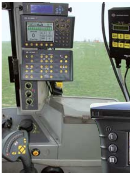
The cab-mounted computer and its joystick. Other control units are for automatic boom section control and boom height control (to the right)...
