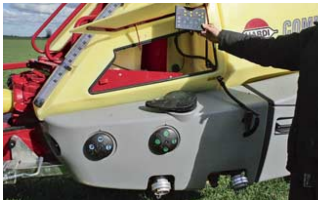
Electric suction and pressure tap controls are duplicated on the external control panel. The digital tank level indicator is the only function that is not controlled from this panel.
